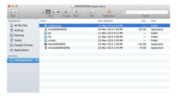
⇒ To install the driver, click **InstallSAM4SJPOS application** in the folder to install the **SAM4S Receipt Printer JPOS Driver.** It will prompt for root user password, enter the root password then click the **OK** button as shown in the following screen to install the SAM4S Receipt printer JPOS driver in Mac OS X.
