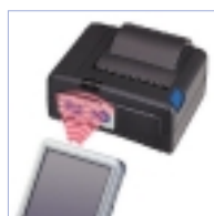
Wireless communication using IrDA
