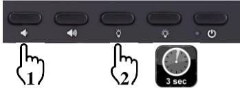
**Press** the Volume Down and Backlight Brightness Down buttons **sequentially and then hold for 3 seconds.**
