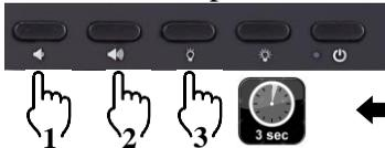
**Press** the Volume Down, Volume Up, and Backlight Brightness Down buttons **sequentially and then hold for 3 seconds.**
