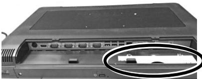
3. Determine to make the USB connector of the dongle be toward the right side.
