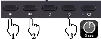
**Press** the Volume Down, Volume Up, and Backlight Brightness Up buttons **sequentially and then hold for 3 seconds.**
