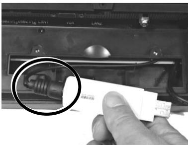
5. Squeeze the coaxial cable connected to the cable TV tuner dongle into the cable TV tuner dongle compartment of the terminal.
