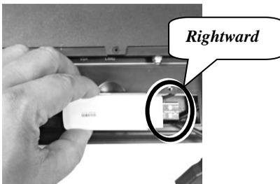
4. Make the connector of coaxial cable extended from the terminal connect to the coaxial cable connect of the cable TV tuner dongle.
