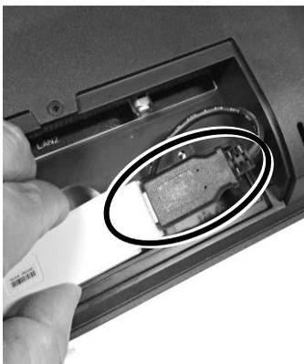
7. Squeeze the USB cable connected to the cable TV tuner dongle into the cable TV tuner dongle compartment of the terminal.
