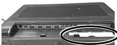
10. Place the I/O port cover back for shielding the I/O ports of the terminal.
