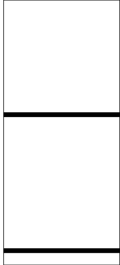
♣ In case of the B/M type media, the black mark must be located in the center of the media because the detect sensor is in the center position of the printer. So the B/M of next 1 and 2 types cannot be detected.
