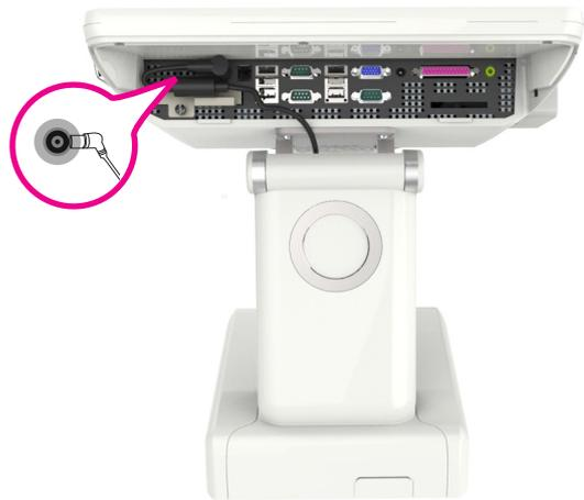
4. As shown in below left picture, remove the screw (1pcs) and the cable cover following the direction of the arrow.
