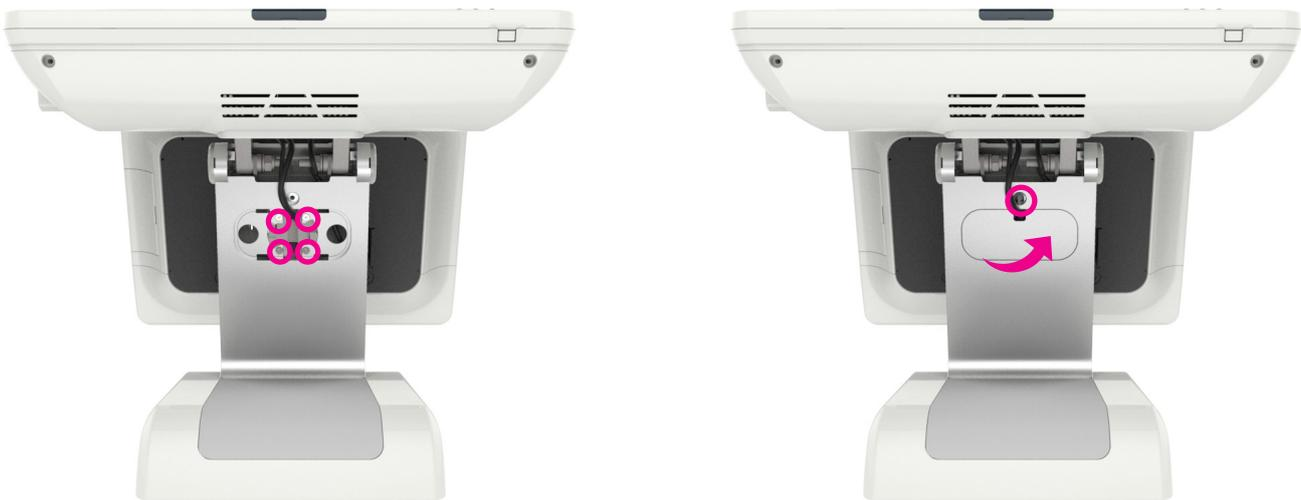
5. Refer to No. 6 of page 25 and connect VGA and power cable and assemble the 'Interface cover.'
