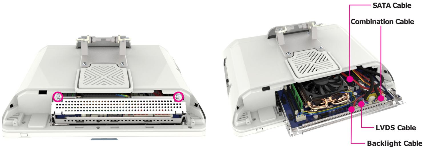
5. Grab on the handle of `Motherboard open bracket' and pull in the direction of below picture and disassemble the motherboard.
