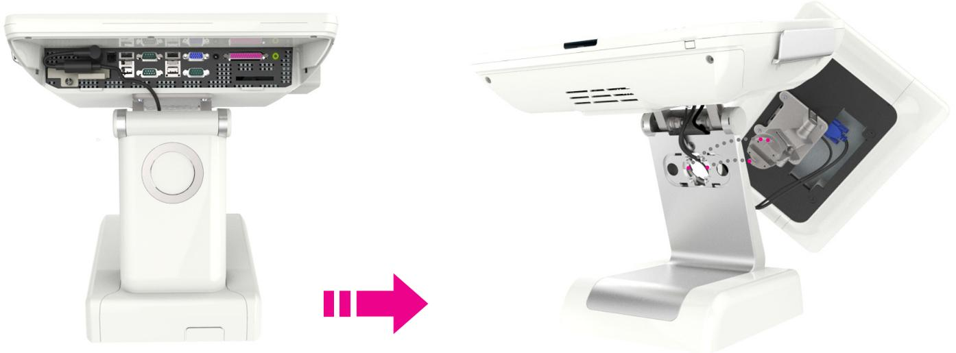
3. Tilt the dual monitor left 45 degrees to arrange the dual monitor in right position.
