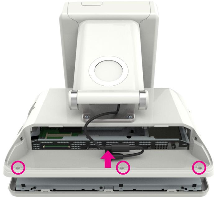
2. Remove the hand screw on the HDD and separate the HDD. (Refer to page 36)
