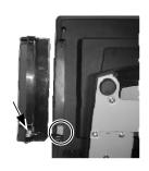
Take out the cable inside this cover as circled in the left picture here and connect it to connector inside the side
