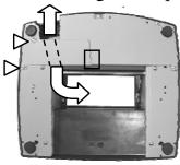
Refer to the bottom view picture of the separated base at left, pass all cable through the dash lined tunnel under a steel plate. Open the steel plate if necessary by removing the 2 triangle marked screws. Insert the rectangular marked end first when reinstalling the steel plate.
