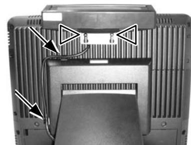
the DC supply in COM port is not required, it will be powered through the USB port.
