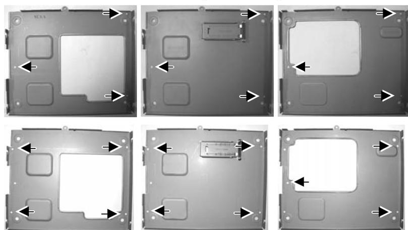
mechanical fixation parts in the wall mount bracket and hang the backpack to the back cover that is already fixed on wall with the cables coming out of the brackets through the openings marked with rectangles in the top row pictures above. Screw lock the top side of the backpack.
