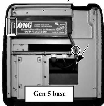
slim base model, please refer to the left picture and place the UPS battery in the cavity in base with the rectangular marked end first. Route the battery connection cable together with all other external connection cables through the arrow marked passage to the battery connector on the main unit. If the optional cable clip is available, insert it into a hole marked in circle in the picture and use it to hold the
