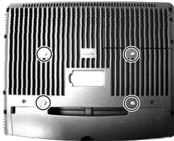
The area required for wall mount application is determined by the main unit dimensions and is 378 mm in width and 312 mm in height for KS-6615/7315 and is 426 mm in width and 370 mm in height for KS-6617/7317.
