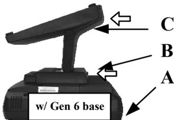
**Step B:** Press the Lock/Release button for main unit detach and meantime ...
