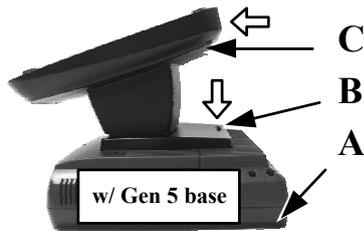
**Step A:** Prepare a soft clean flat surface, such as a piece of cloth on the desk to seat the front surface of main unit after being adjusted to most horizontal position
