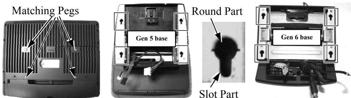
Match the matching pegs on the back of the main unit against the (rectangular marked above for both base types) matching holes on the stand assembly. First aim the matching pegs toward the upper round part of the hole (ref. the close-up illustration) and make sure that all pegs are inside the holes.
