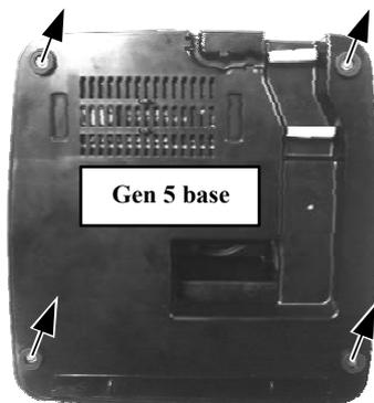
Take the adjustable stand assembly of the gen 5 slim base and turn it up side down to show the bottom of the base. Remove the bottom plate fixing screws in center of rubber feet to remove the bottom plate. For maintenance operation that there are already some cable connections, please release the cables from the 2 plastic cable holders and have all cables to pass through the cable passage in bottom plate as in the left picture.
