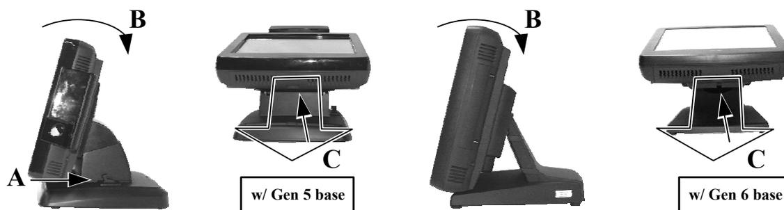
**Step A:** Push lock/release lever of the Gen 5 slim base for tilt angle adjust backward. (This operation is not required in Gen 6 super slim base)
