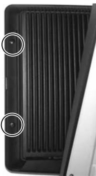
Remove the 2 screws circled in the left picture to remove the cover for side mount upgrade kit. Take out the cable inside this cover and connect it to the white connector inside the side mount upgrade kit like SD-680 as arrowed in the right picture. Gently arrange the excessive length of this cable back in the hole and screw-fit it back to
