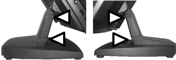
the side view pictures of the base trunk at the left and release the triangle marked hooks to remove the back cover.
