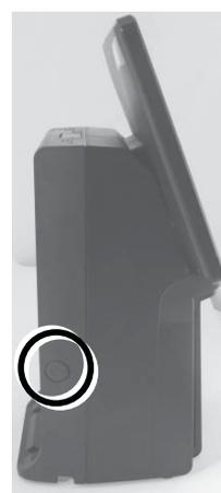
If the system hangs due to a reason, such as software resource conflict, please press and hold the power button for over 10 seconds around to forcedly shut down the system.
