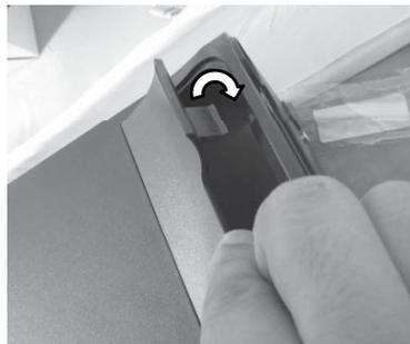
8. Determine that the I/O interface is covered and the cable passes through the cable exit.
