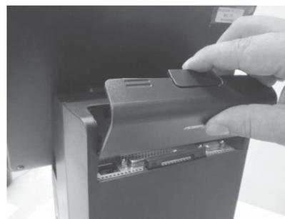
4. Connect I/O cables to the top I/O interface of the desktop POS and then gather the cables together in the cable exit.
