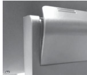
8. Push the cover to make the 2 hooks of the cover to wedge the 2 wedge portions of the rear plate of the POS.
