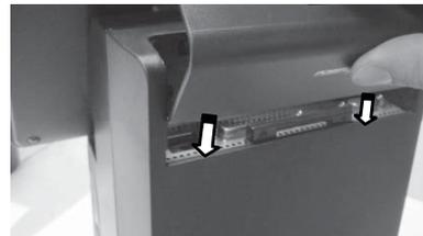
7. Determine that the cover is well wedged to the wedge portions of the rear plate of the POS.
