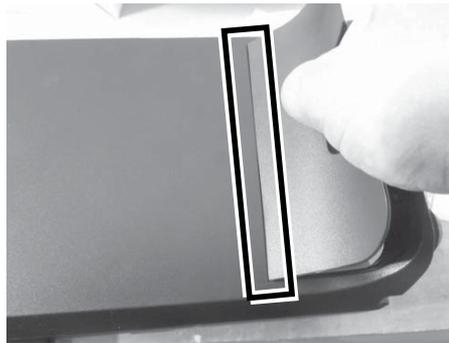
7. Gather the I/O cables together for cable arrangement and lever down the 2 hooks of the cover to cover the I/O interface.
