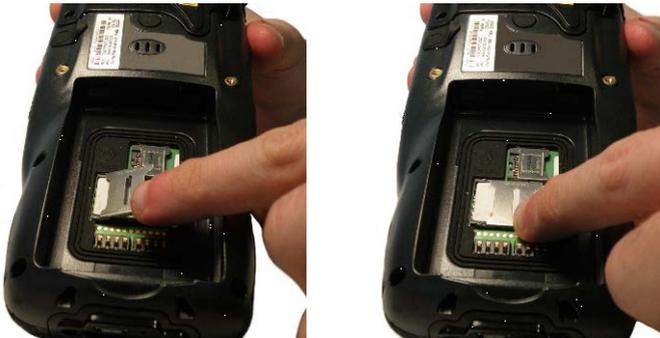
6. First insert the bottom and then the upper (contacts) side of the battery pack into the slot. First insert the bottom and then the upper (contacts) side of the battery pack into the slot. Press until the battery latch clicks twice.
