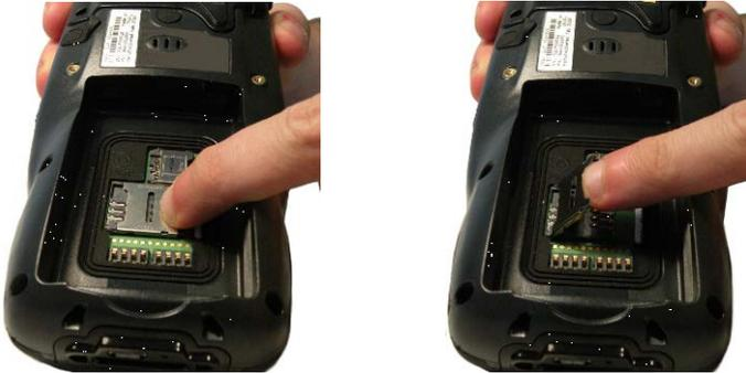
4. Insert the SIM card with the contacts downward:
