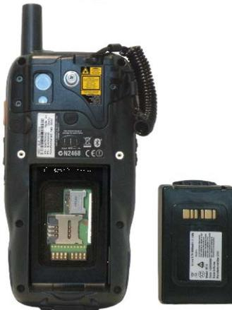
4. Install the new battery pack, first insert the bottom side, then the upper (contacts) side of the battery pack into the slot. Press until the battery latch clicks twice:
