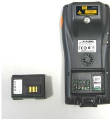
4. Replace the battery pack by pressing the latch release button and pulling the battery latch down, and then by inserting it towards the speaker and pressing it into the Datalogic J Series™ PDA until the battery latch is automatically closed:
