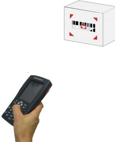
The Datalogic J Series™ Imager uses an intelligent aiming system pattern, similar to those on cameras, indicating the field of view, which should be positioned over the code:
