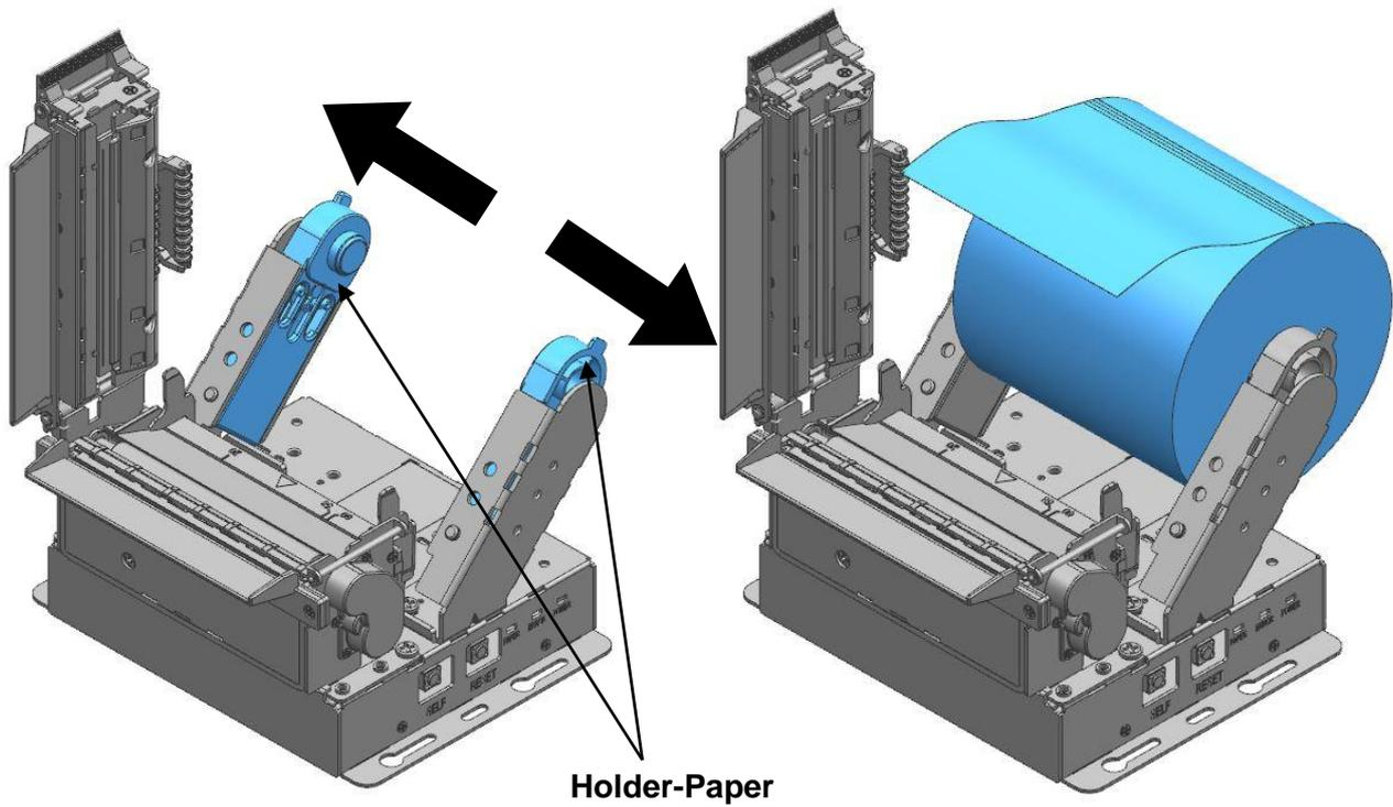
Check the orientation of the roll paper when inserting it into the printer.
