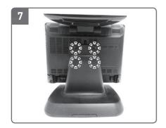
Assemble stand and install 4 screws.
