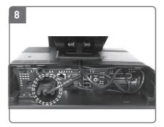
Connect RGB cable of monitor to the DC Out port on connection panel.
