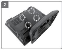
Lay terminal face down on a soft surface. Remove 4 screws as shown.
