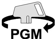
S. This position should only be used by programmers, engineers or other people trained to carry out tests or programming functions
