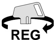
Register position. This is the normal working position. The key can be removed whilst the lock is in this position
