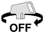
Off position. The register is still working but the keyboard is disabled. The key can be removed whilst the lock is in this position.
