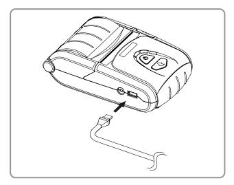
1) Connect the interface cable (optional) to the cable connector of the printer.
