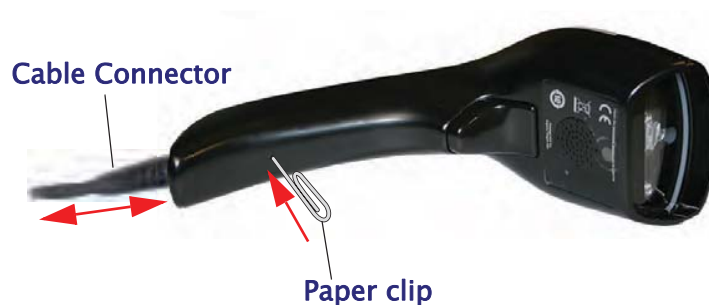
Figure 2. Cable Connection/Disconnection at the Scanner
