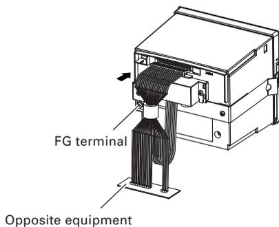
5. Connect the printer FG terminal to ground. Be sure to make this connection to prevent noise, static charge, etc. Firmly make this connection using the terminal screw at the rear of the printer.
