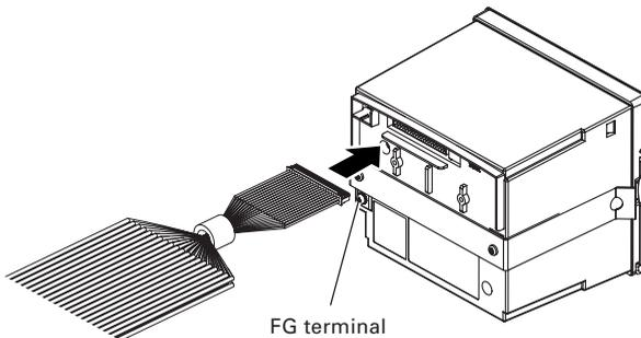
5. Connect the printer FG terminal to ground. Be sure to make this connection to prevent noise, static charge, etc. Firmly make this connection using the terminal screw at the rear of the printer.
