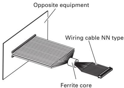
4. After making sure the printer power is OFF, orient the connector correctly and firmly connect it to the printer.
