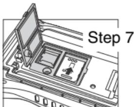
8. Lift the door up to expose the socket.
