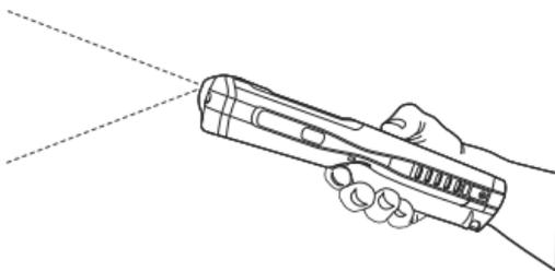
3. Project the aiming beam or pattern by pressing and holding the SCAN key
