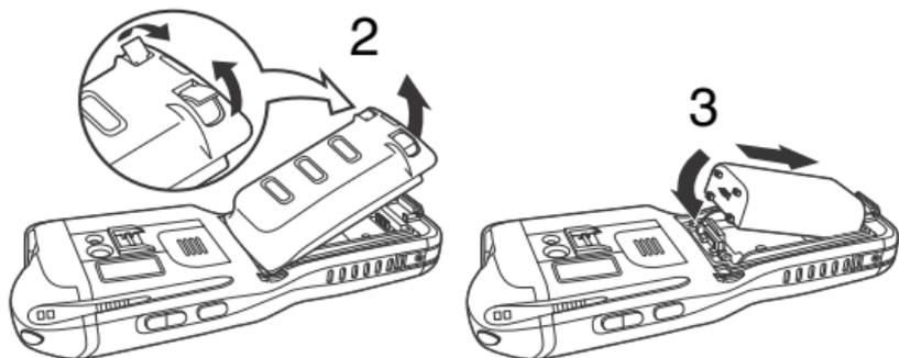
4. Replace the battery door. Apply pressure to engage the door latch. The battery door must be installed prior to powering the unit.
