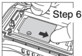
7. Unlock the access door to the socket by sliding the door toward the IrDA port side of the terminal.
