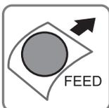
Use this button to feed paper or to start self test and for hexadecimal dump mode. (See the instructions "Self test" (2.2.3) in this chapter for self test.) (See the instructions "Hexadecimal dump" (2.2.4) in Chapter 2 for hexadecimal dump mode.)
