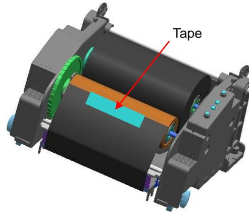
(4) Press the Close area to shut the ribbon assembly.
