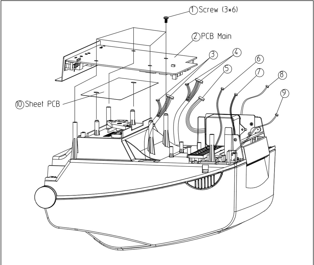
**Figure 5-2 Disassembly Case-Lower #2**
