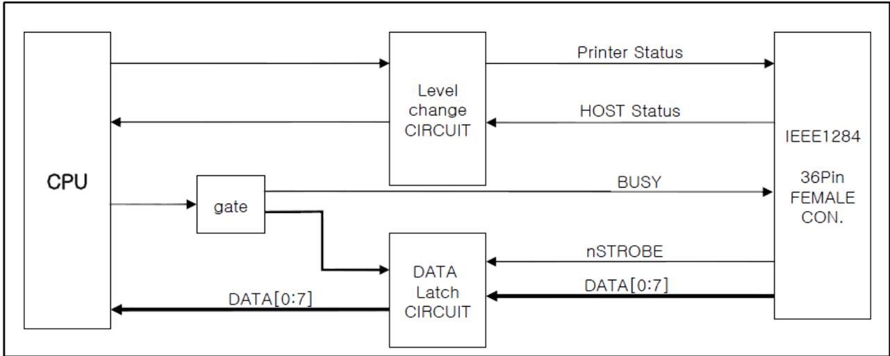
**Figure 4-4 IEEE1284 Communication Block Diagram**
