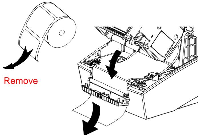
5) Adjust the paper guides and close the label peel-off cover.
