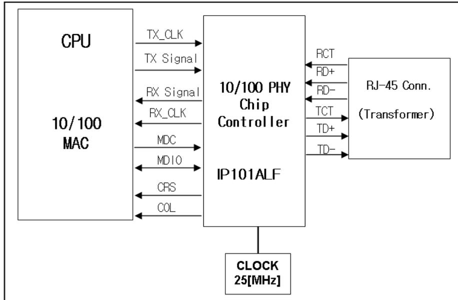
**Figure 4-6 Ethernet Communication Block Diagram**
