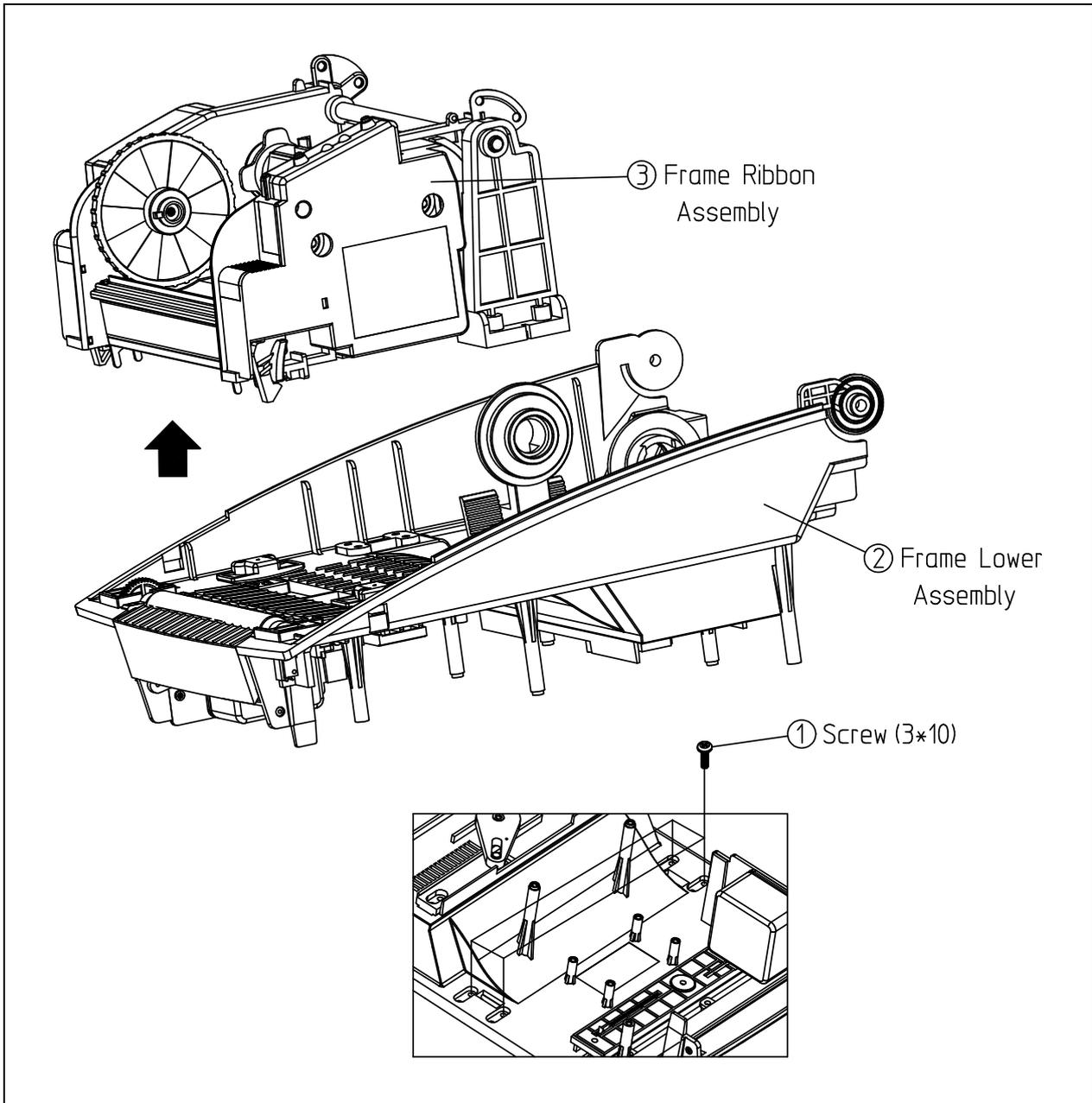
**Figure 5-4 Disassembly Frame Ribbon #1**
