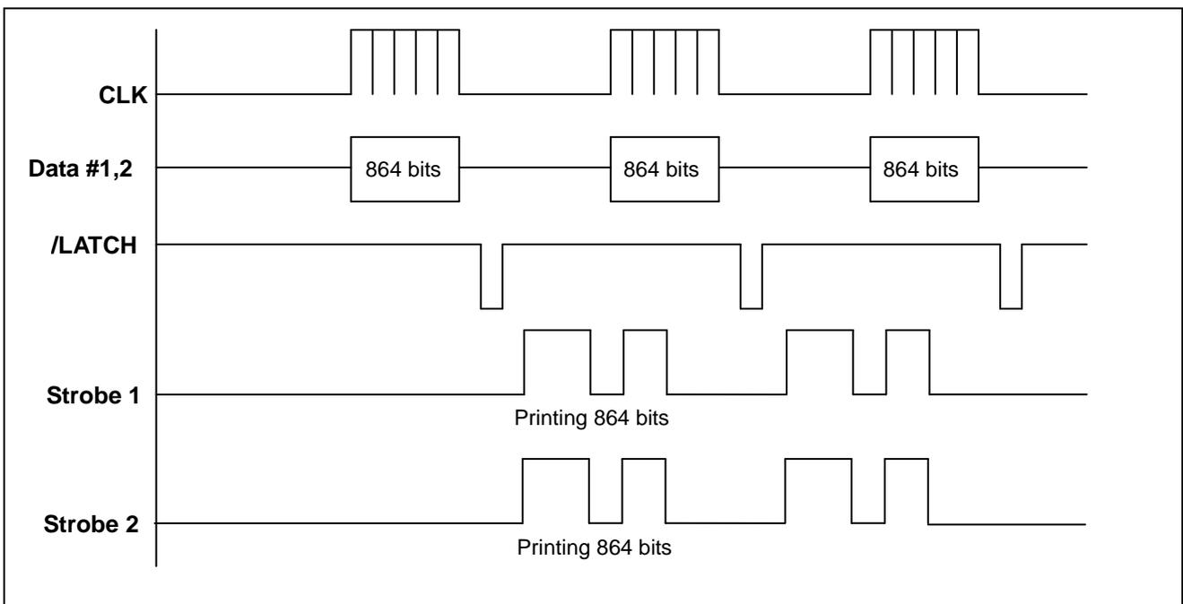
**Figure 4-8 Thermal Printer Timing Waveform**
