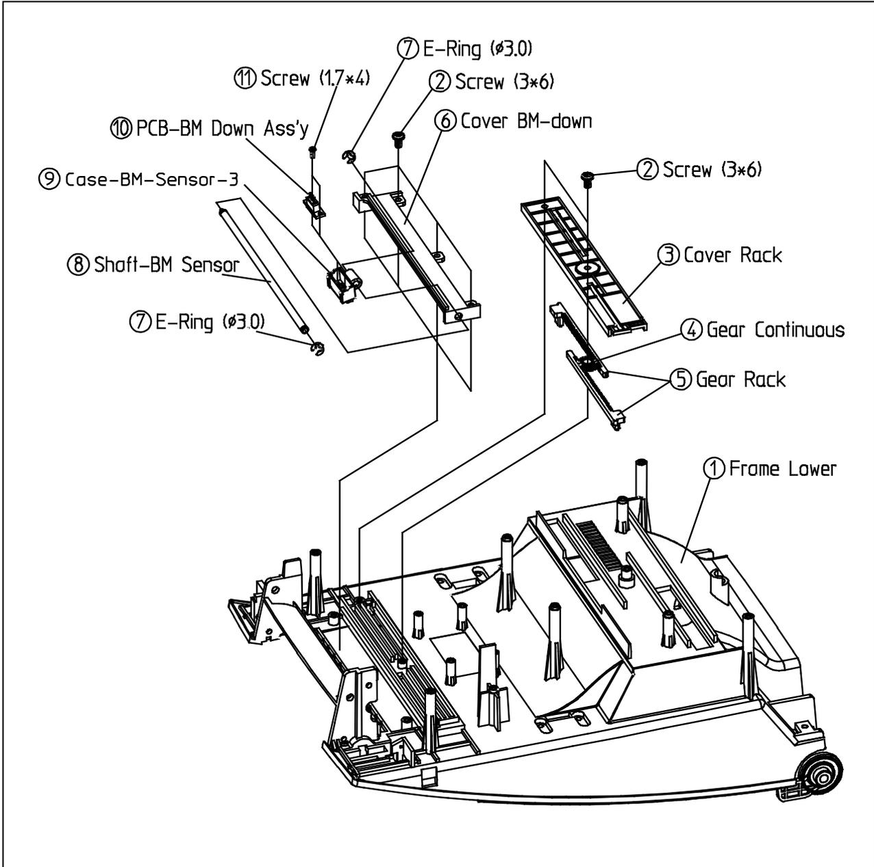
**Figure 5-13 Disassembly Frame Lower #4**
