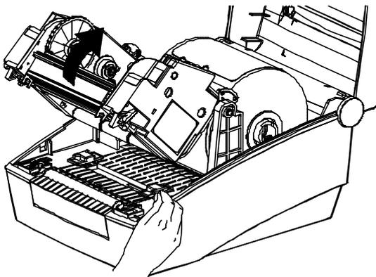
4) Feed the paper between the Paper Guide on both sides.
