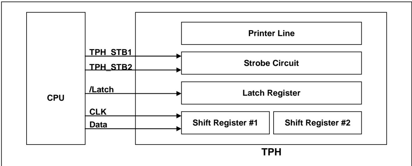
**Figure 4-7 Thermal Printer Block Diagram**
