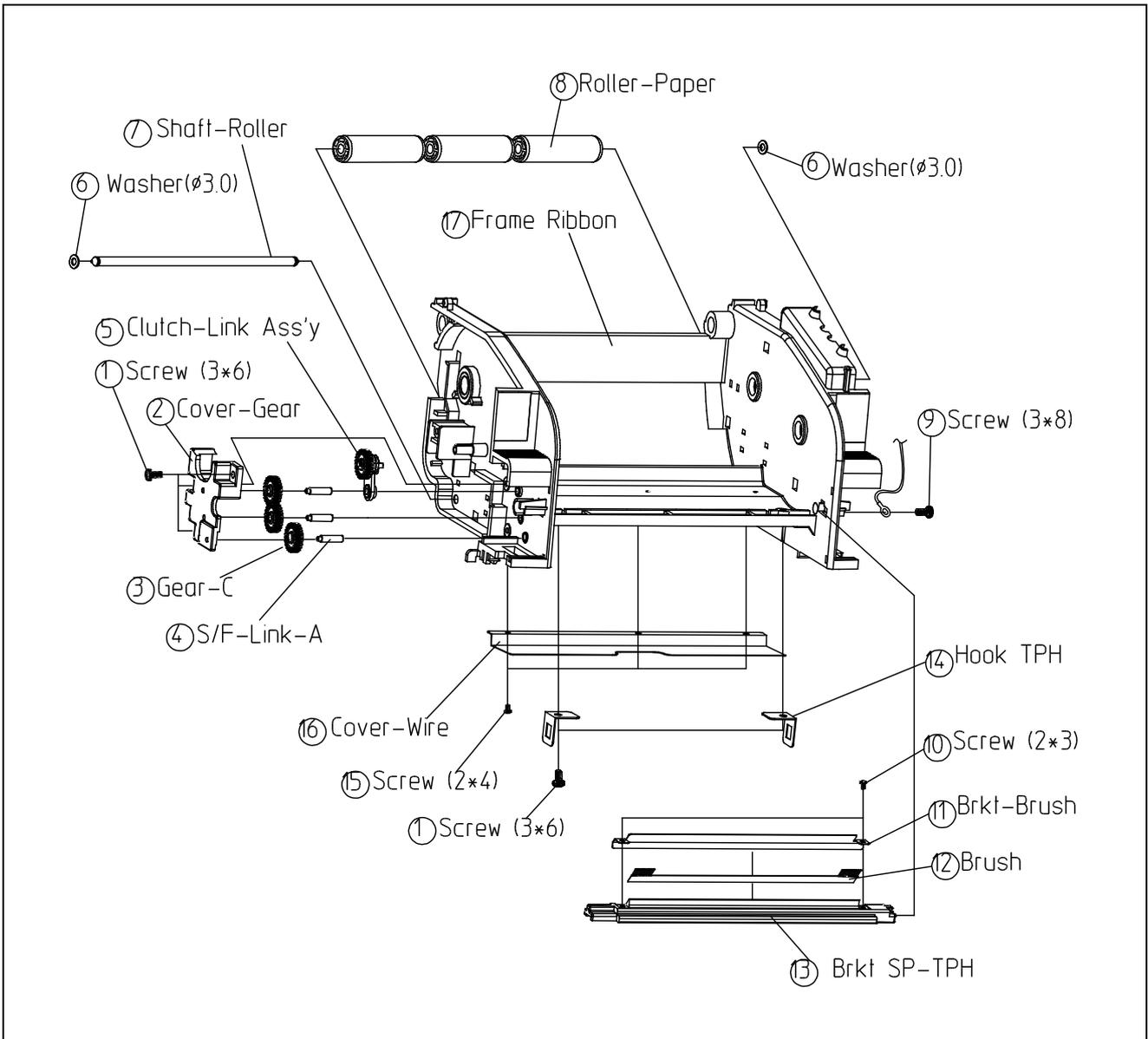
**Figure 5-9 Disassembly Frame Ribbon #6**
