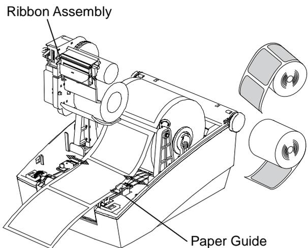
5) After Installation the paper, manually set the sensor(Gap & Black-Mark) and Paper Guide to the correct position.
