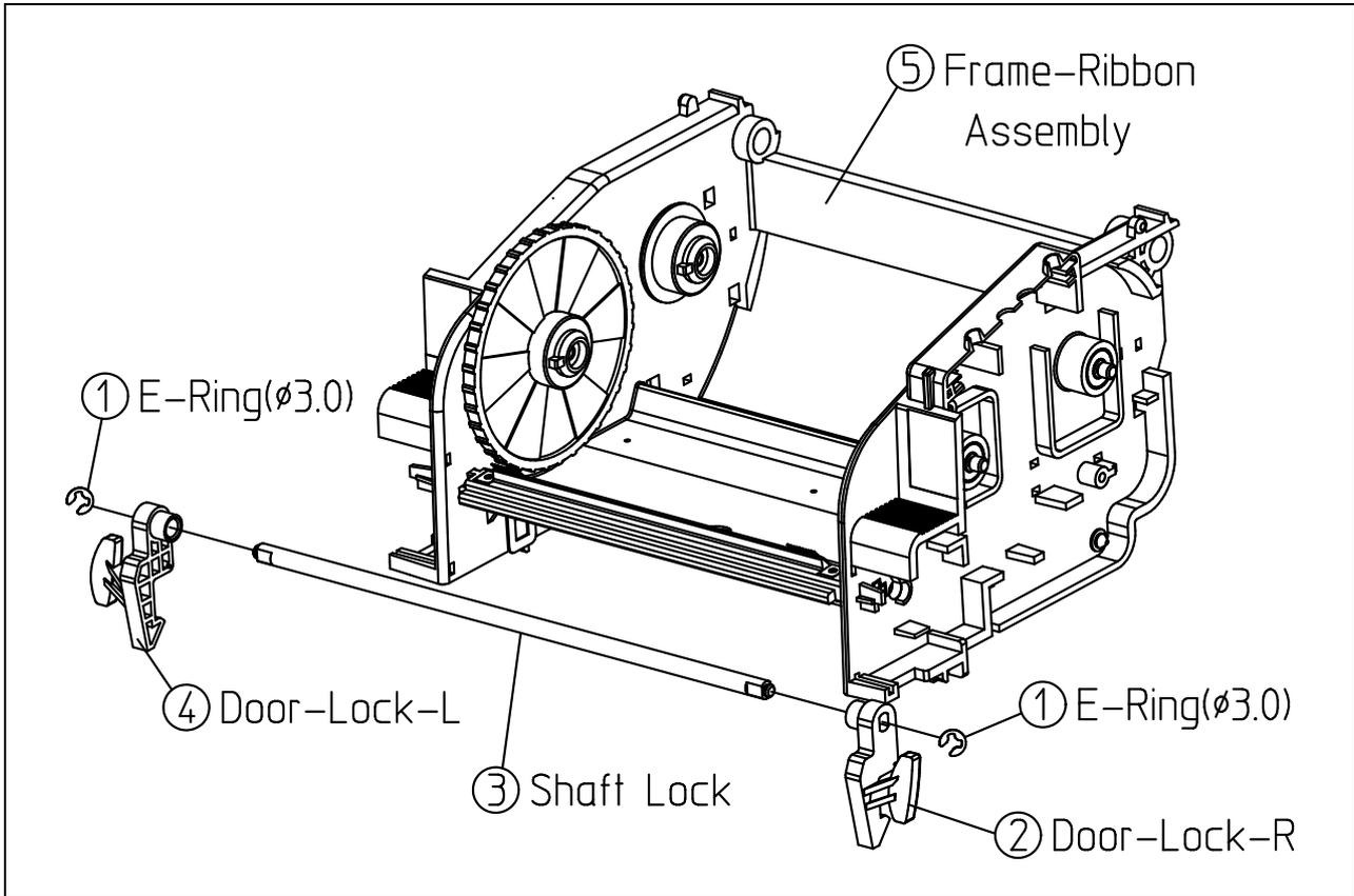
**Figure 5-7 Disassembly Frame Ribbon #4**
