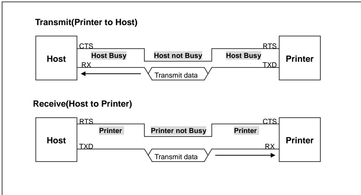
Figure 4-3 RS232C Communication Waveform
