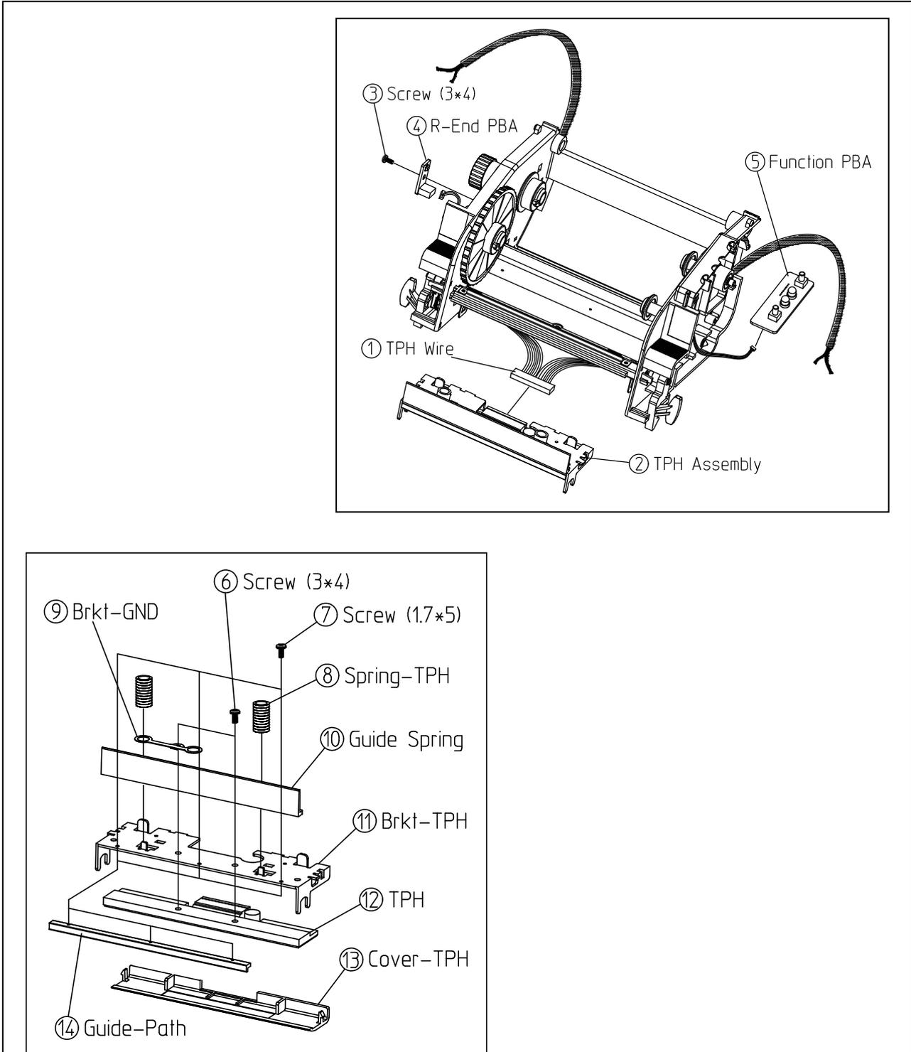
**Figure 5-6 Disassembly Frame Ribbon #3**
