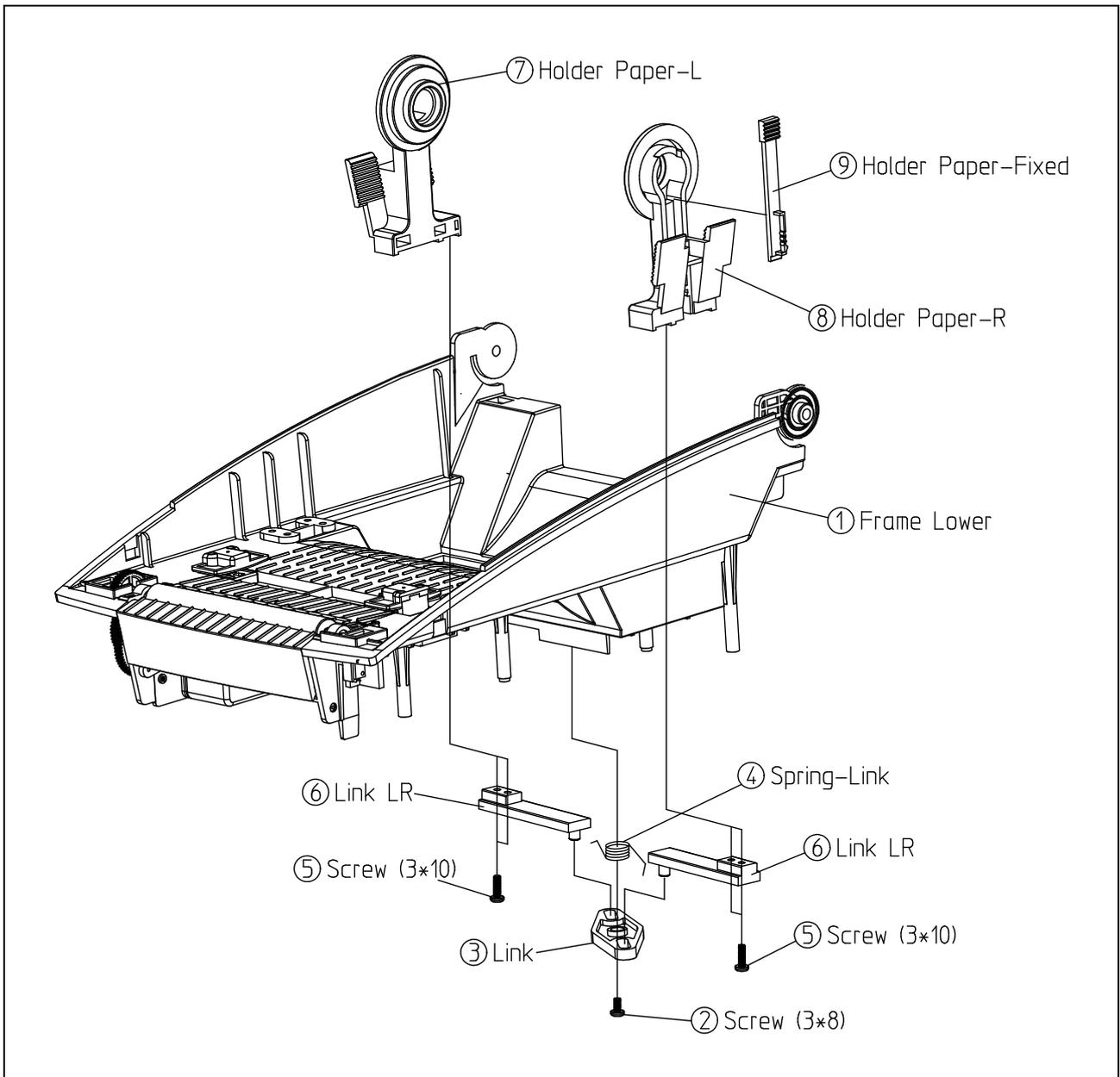
**Figure 5-10 Disassembly Frame Lower #1**
