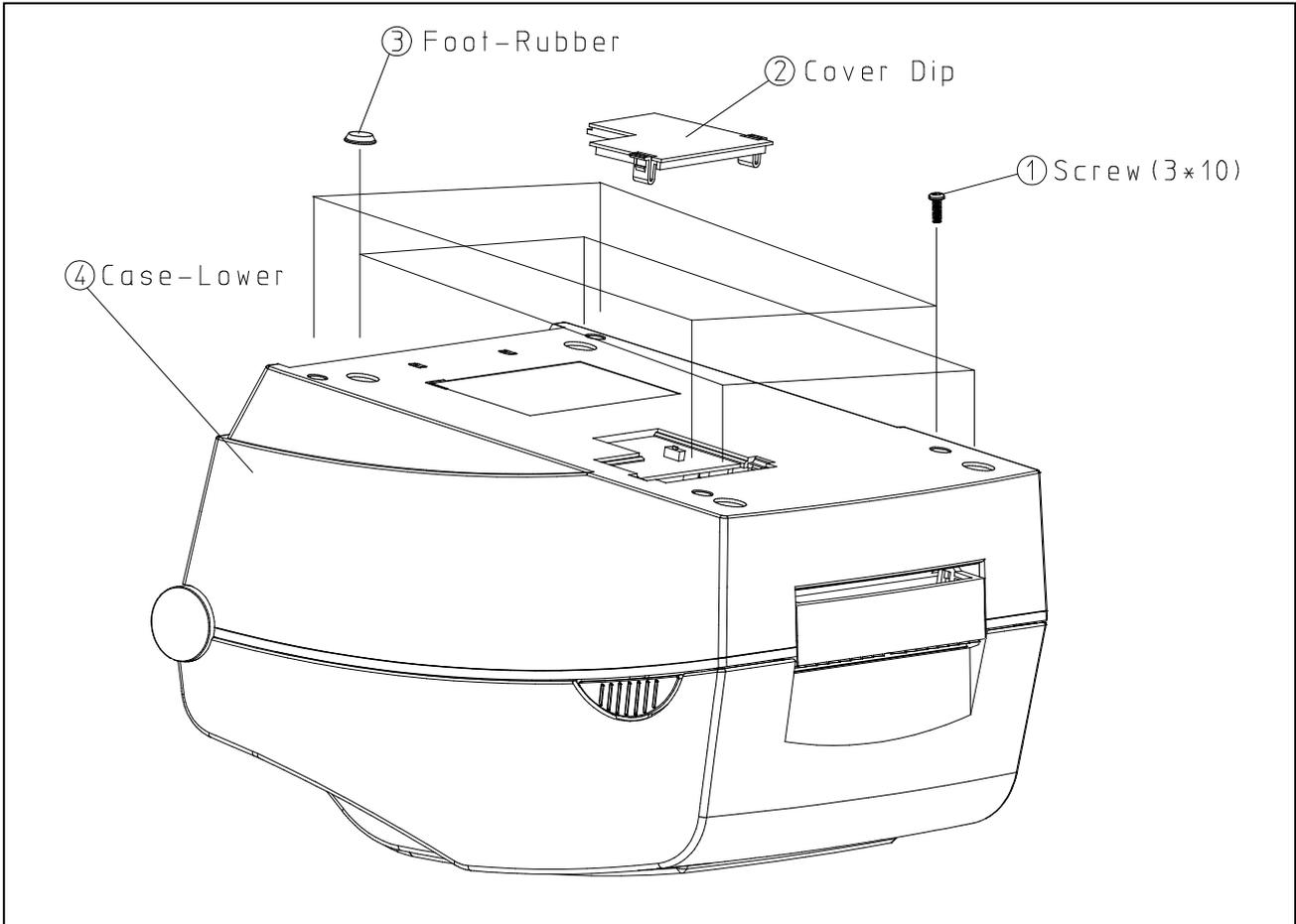
**Figure 5-1 Disassembly Case-Lower #1**
