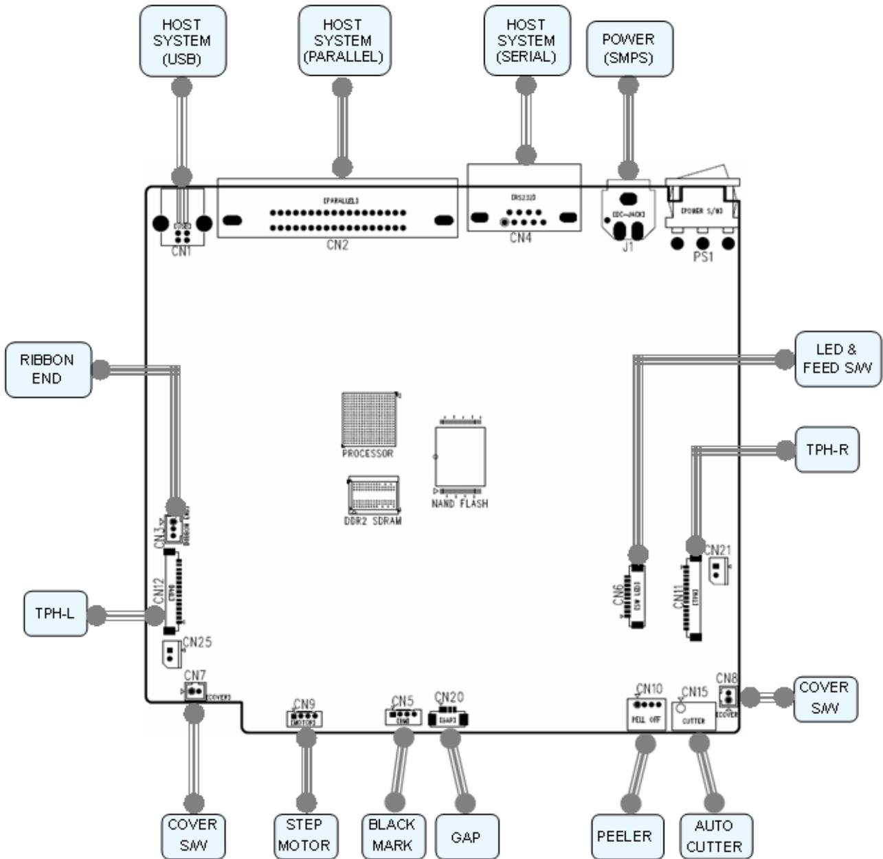
**4-1-2 SLP-TX40xE Board Wiring Diagram**
