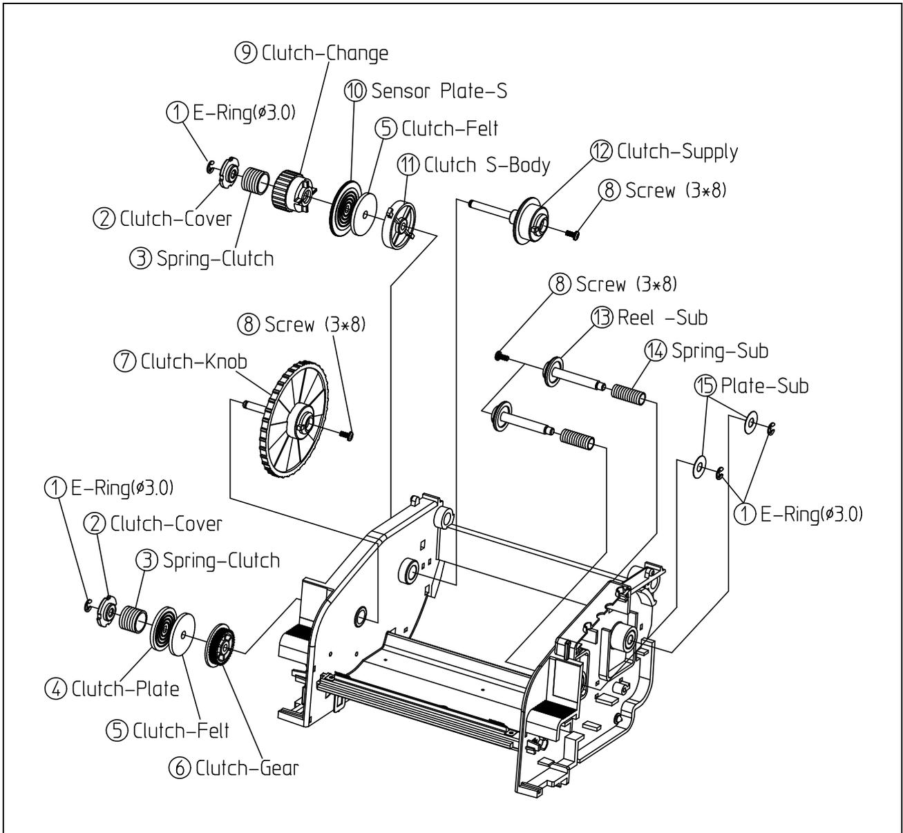
**Figure 5-8 Disassembly Frame Ribbon #5**
