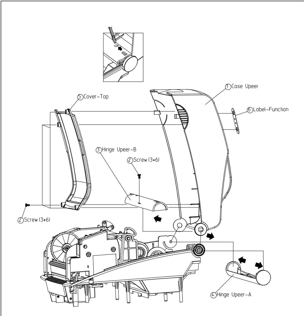
**Figure 5-3 Disassembly Case Upper #1**
