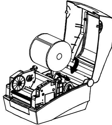
3) Open the Ribbon Assembly and spread the paper guide.
