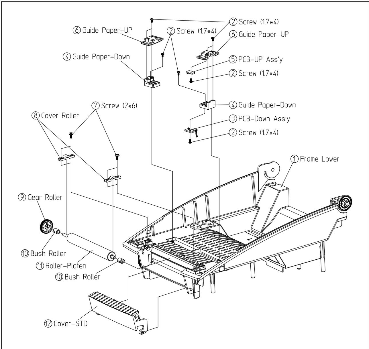
**Figure 5-11 Disassembly Frame Lower #2**
