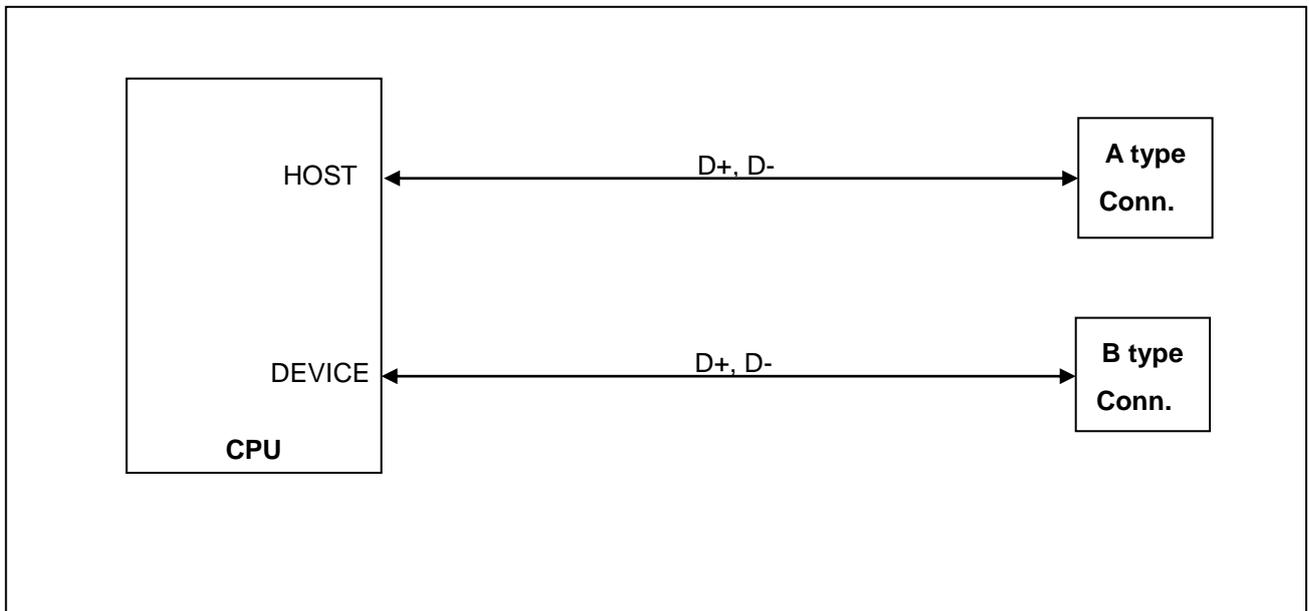
**Figure 4-5 USB 2.0 Communication Block Diagram**
