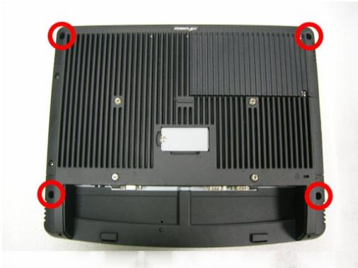
Separate the panel assembly and the main unit by unfastening 4 screws as indicated.
