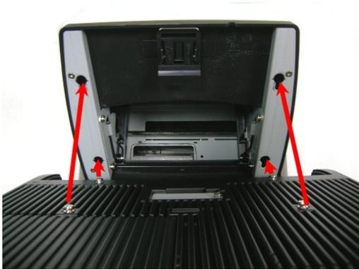
Lineup 4 studs on the back of the main unit to the 4 holes on the base stand, and then install the main unit to the base stand.
