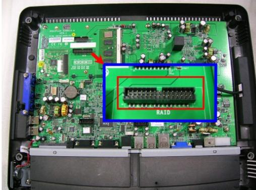
Remove all the Jumper caps from the RAID control board connector on the M/B.
