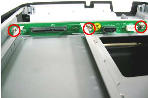
Install the SATA HDD extension board to the base stand. Fasten it in place with 3 \* (#6/32-6L+SW) screws.
