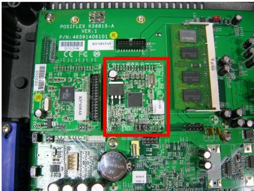
Install the RAID control board.
