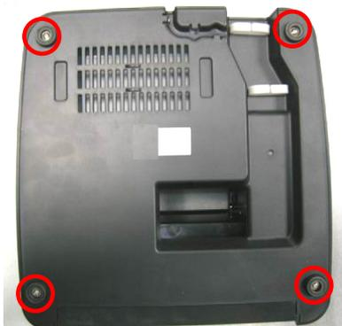
Close the bottom cover, and then fasten it with 4 screws.
