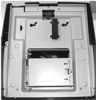
protected devices to a Gen 4 slim base or Gen 5 slim base include: a 2.5" system HDD and an optional UPS battery
