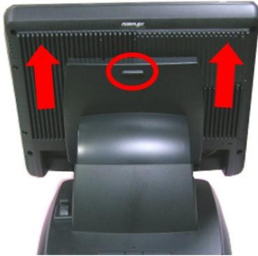
Press the Release Button, and then lift up the main unit as shown in the picture.
