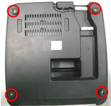
Unfasten the 4 screws to remove the bottom cover.
