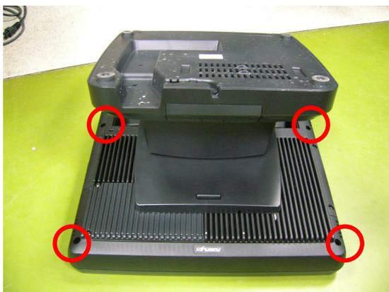
Shut down the system. Fasten the Panel Assembly to the main unit with 4 screws.
