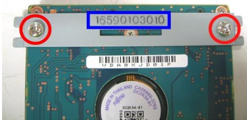
Fasten the HDD bracket to the 2<sup>nd</sup> HDD with 2 screws. Make sure the bracket is right way round; the numbers should be in the top as shown in the picture.
