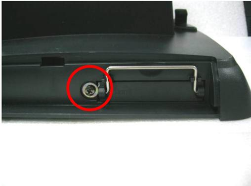
Fasten the HDD module with the screw,
