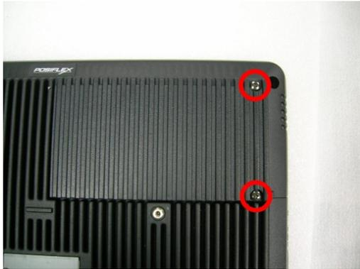
Unfasten the HDD cover by removing 2 screws.
