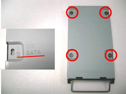
Install the HDD removed from the main unit to the HDD bracket for the base stand. Fasten it with 4 screws. Make sure the screw hole for SATA is used.
