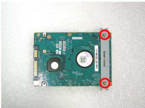
Remove the HDD bracket by unfastening the 2 screws.
