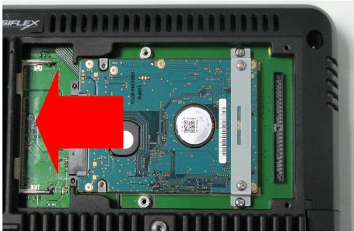
Inside the HDD cover, there is a DDR2 SODIMM socket for memory expansion which is near by the HDD. Please note the supported memory type specified in the earlier chapter GENERAL SPECIFICATIONS if upgrade or replacement is required.
