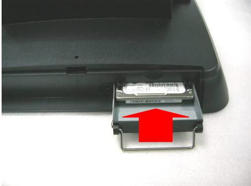
Slide the HDD module into the base stand.
