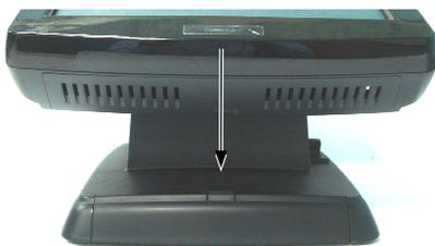
Press down the arrowed center part of the front cover in the base to remove the front cover as indicated in the left picture. Should there be difficulty removing it, please check if there is any locking screw nearby the center part of the cover.
