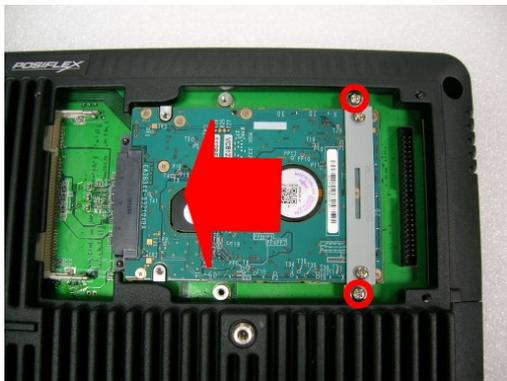
Slide and connect the 2<sup>nd</sup> HDD + bracket in place as shown in the picture, and then fasten it with 2 screws.
