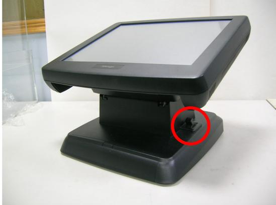
Push the gear lever on the base stand to flatten the main unit.
