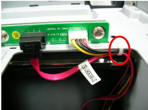
Connect the SATA HDD cable to the extension board, and then fix it with a cable tie (if one is available).
