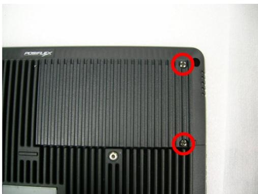
Close the HDD cover, and then fasten it with 2 screws.
