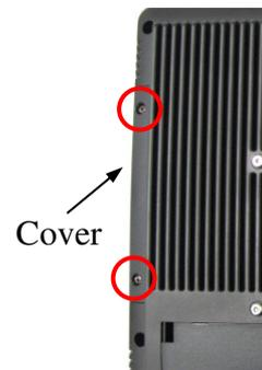
open the cover, connect the cable found inside the cover to the side mount unit then align the side mount unit on the right edge of the main unit and fasten the two screws with washer.
